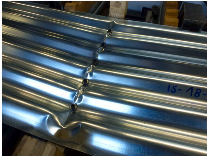
Fig. 17. Failure mode, IS-18-V-063-40-1 (buckling in the crest).
