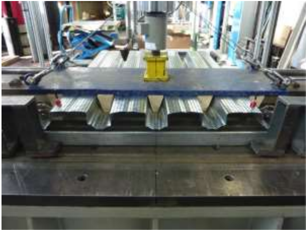
Figure 1.3.8 – End support test on profile with total perforation
