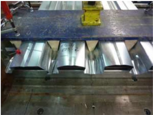
Figure 1.3.5 – End support test on profile without perforation
