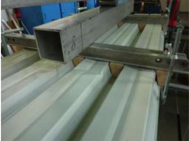
Figure 1.3.1 – Single span test on profile without perforation
