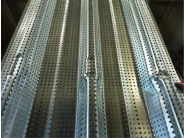
Figure 1.3.12 – Profile with total perforation after internal support testing
