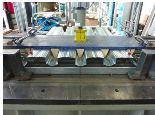
Figure D.11: Web-crippling (exemplary for ES-4l-075-1)
