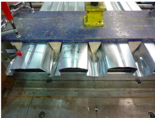
Figure D.7: Web-crippling (exemplary for ES-4-075-2)
