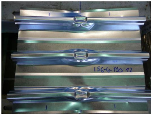
Figure C.13: Failure mode (exemplary for IS6-4-100-12)
