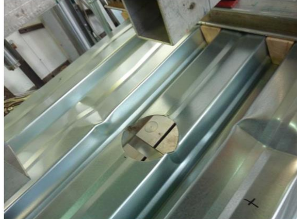
Figure B.10: Failure mode (exemplary for PF-4Hc1-075-2)
