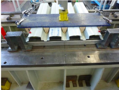
Figure D.10: Web-crippling (exemplary for ES-4w-075-1)
