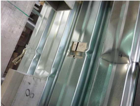
Figure B.9: Failure mode (exemplary for PF-4Hs3-075-1)
